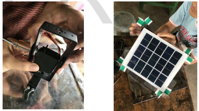
Figure 13. Screwing Servos and Fitting Four LDRs at Coners
